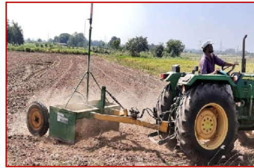
Land levelling with laser guided leveler.
